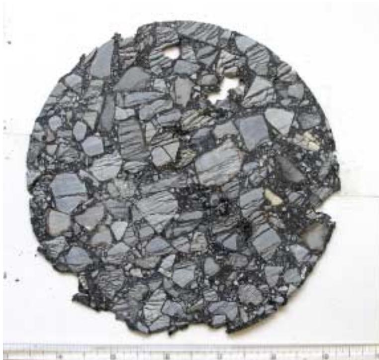
**Picture 13 – Fractured Aggregate (Mat Interior)**
